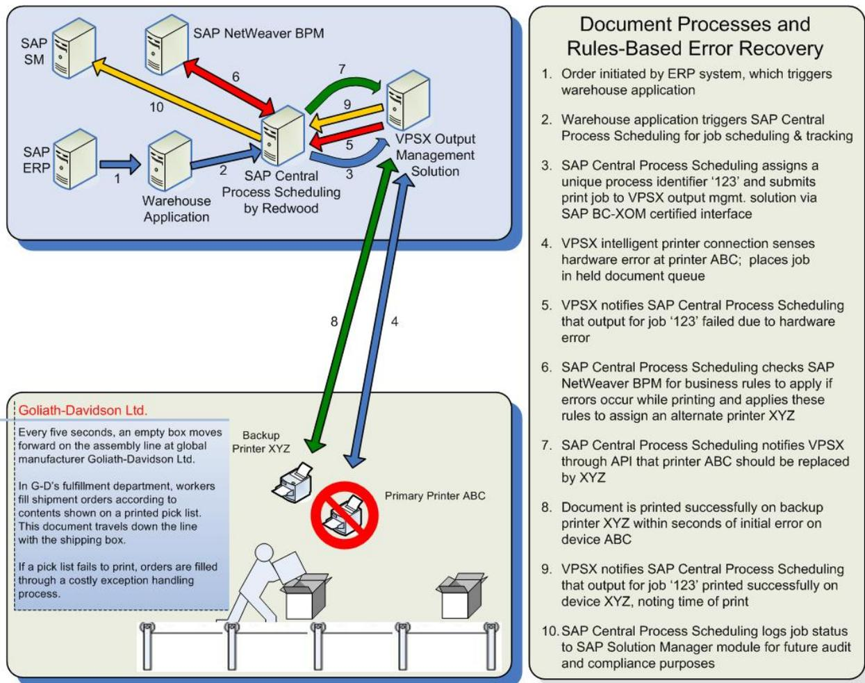
As complex electromechanical devices, printers are prone to a variety of failures — paper jams, missing/low toner and other supplies, loose connectors, etc. Intelligent output management solutions like VPSX software instantly sense such conditions and trigger appropriate action. Such solutions serve as both the vanguard of business process continuity and the “eyes and ears” for SAP NetWeaver Business Process Management (SAP NetWeaver BPM), SAP Solution Manager, and the like.
